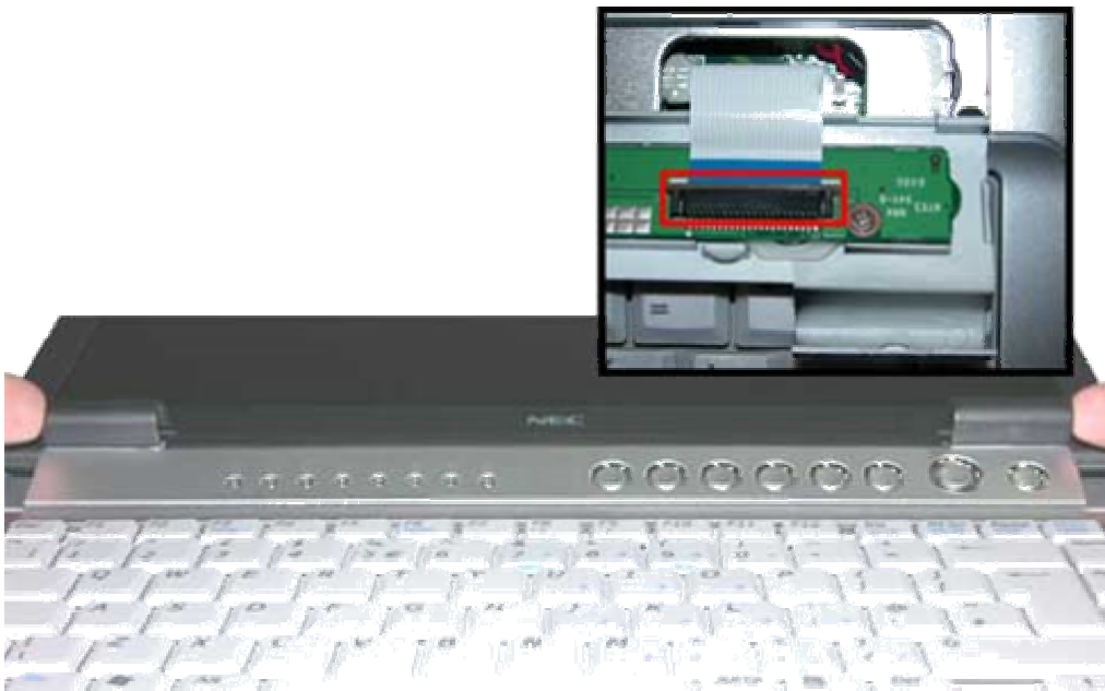
Fig. 8 Lifting up the Keyboard Cover
